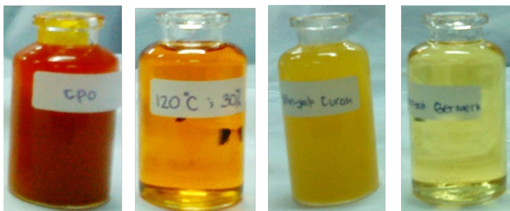
Figure 6. Physical Appearance of Palm Oil: (a) CPO, (b) Resulting from Bleaching with Pumice at Optimum Condition (Temperature of 120 °C and Bleacher Content of 30%), (c) Bulk Cooking Oil, (d) Branded Cooking Oil
