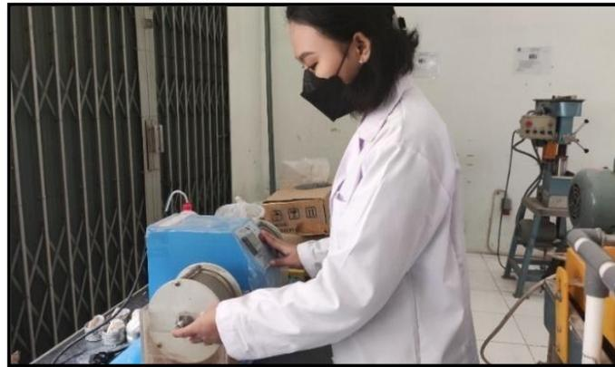
**Gambar 1.** Pengujian *Slake Durability*
