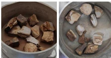
**Gambar 10.** Hasil Pengujian *Durability* Sampel 7
