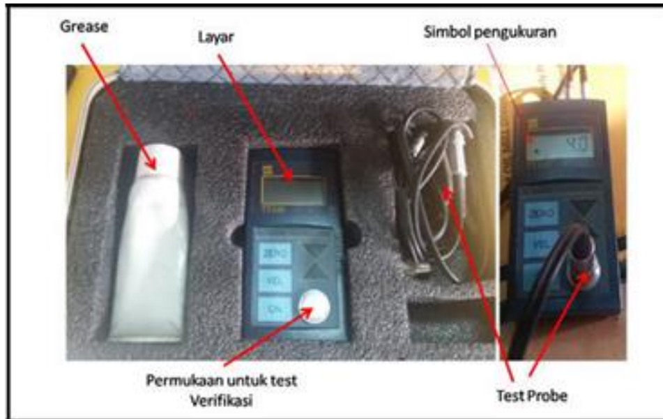
Gambar 1. Smart Sensor Ultrasonic Thickness Gauge TT 130
